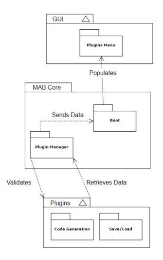
Fig 4: Architecture of the Plugin Framework
